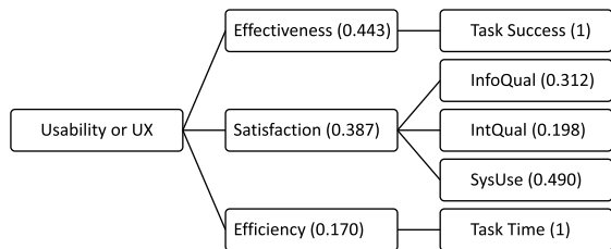
Fig. 1. A hierarchy structure of the evaluated indexes for usability measure (SysUse = System Usefulness, InfoQual = Information Quality, IntQual = Interface Quality).
