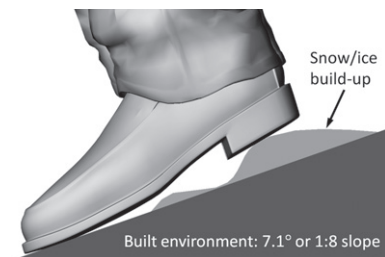
Fig. 6. Snow/ice build-up can increase the effective slope of the built environment.
