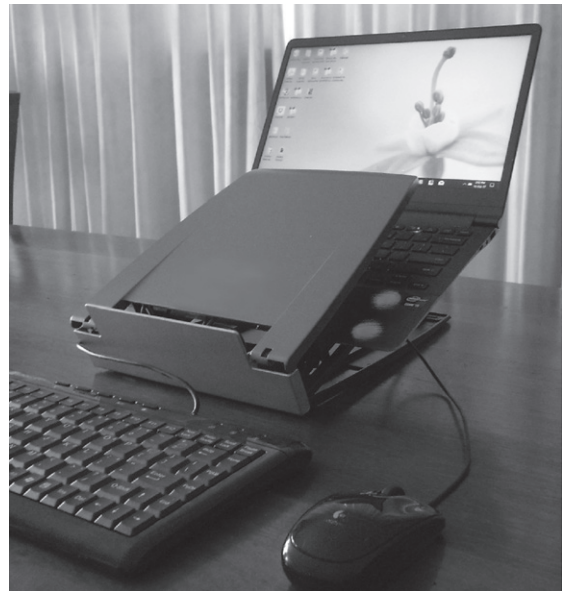
Fig. 3. A laptop stand will raise the height of the monitor so that you don't need to flex your head forward to read from the display. Using an external mouse and keyboard can help your arms and shoulders remain comfortable.
