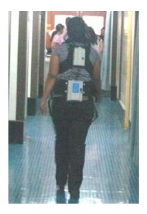
Fig 1: Recording of lumbar kinematics by iLMM
