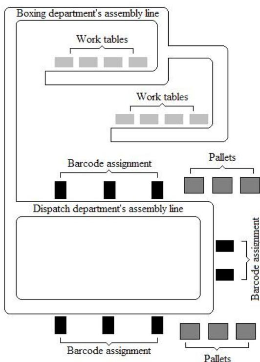
Fig. 2 - Boxing and dispatch departments' assembly line configuration after the intervention
