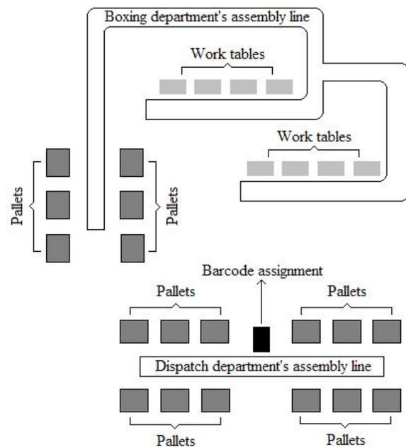
Fig. 1 - Boxing and dispatch departments' assembly line configuration before the intervention
