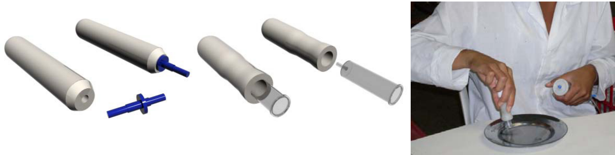
Fig. 03: Manual tool developed (white) and product component blue and transparent. And operator using the tool (right)
