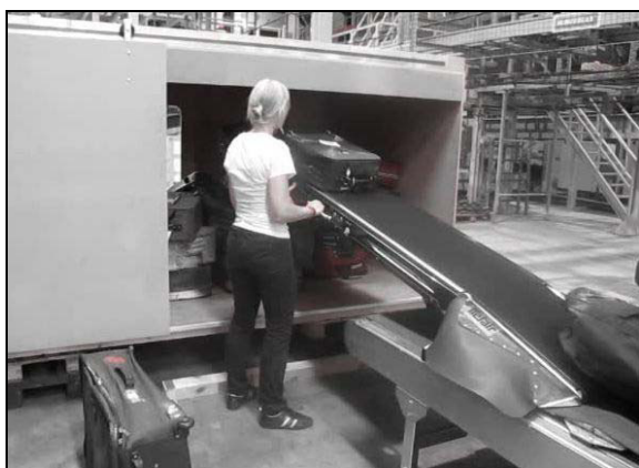
Figure 4: Loading a mock up with a Telair RTT semi-automated loading device.
