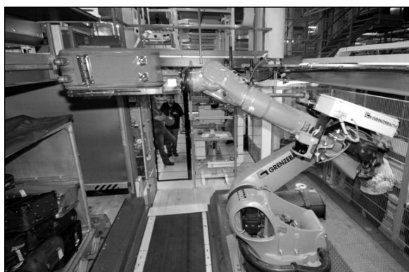
Figure 5: Automated loading of bags (Robot loading)
