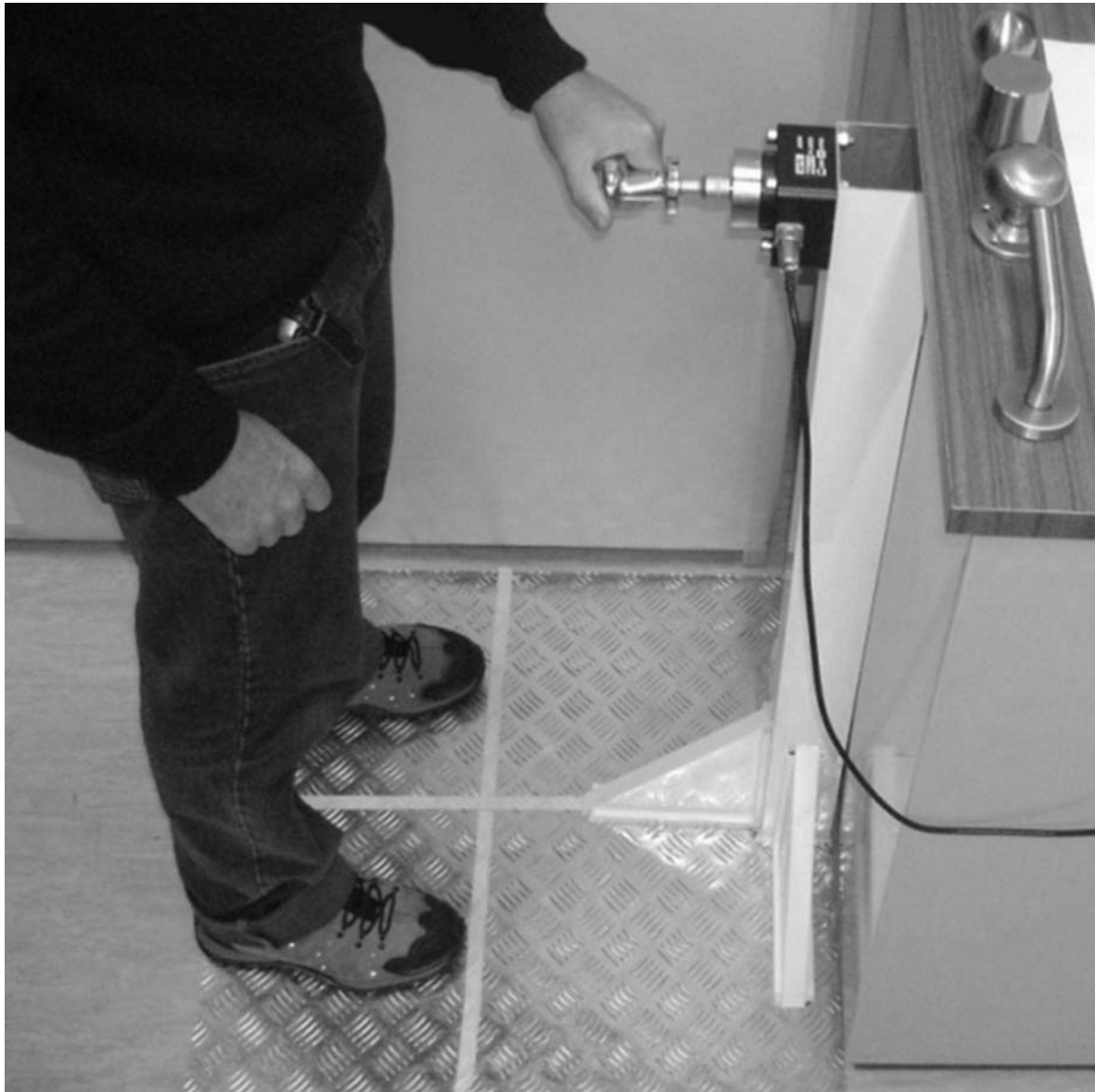
Figure 1. Realization of task simulation in the fixed support used to place the door handles.
