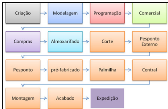
Fig. 2: Production process flowchart in PV. In each box is written: creation, modeling, programming, commercial, purchasing, warehouse, cutting, external stitching, stitching, prefabricated, insole, central, assembly, finishing and shipping respectively
