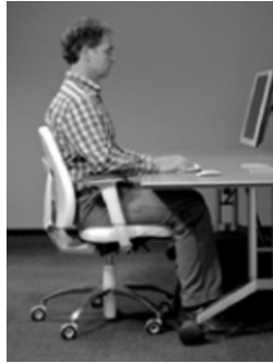
Fig. 1 The percentage of time that was spent in the basic posture can be measured by means of the chair. Feedback about the posture that was adopted during one hour is presented by means of a label on the seat.
