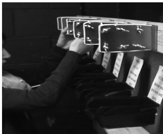
Fig. 1 Assembly at above shoulder height
