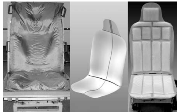
Fig. 2. Three stages in the seat development of the light weight seat: measuring the human contour (left), the CATIA 3d model (middle), the seat shell with inflatable cushions (right).
