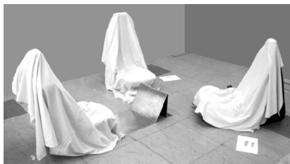
Fig. 3. The test set up for with blankets to prevent that the subjects see the chair.
