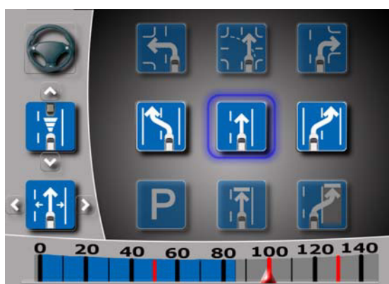
Figure 3: Displayed content of the tactile touch display. In this example two maneuvers are available (“lane change right / left”) and the maneuver “follow lane” is executed.
