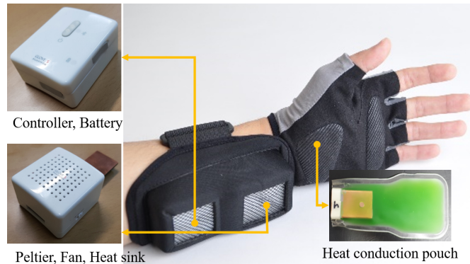
Fig. 1. The customized cooling gloves consisted of a fingerless glove, a heat conduction pouch, a controller and battery pack, a Peltier module with a fan and heat sink, and a wrist pouch.
