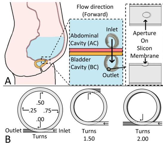
Fig. 1. The newly-designed implantable catheters with silicone apertures to prevent backflow. A: the expected implanting position of the catheter and its features B: the definition of ‘turns.’
