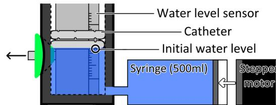
Fig. 2. Experimental setup to test the designed catheters. The initial water level of the experiments was at the lowest located aperture.
