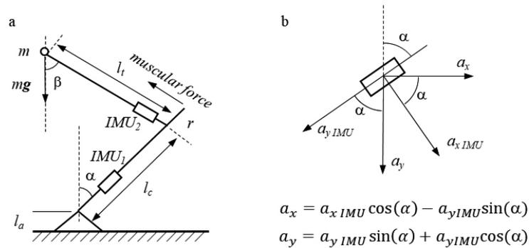
Fig. 3. Geometry of the leg model for the squat exercise (a); the relation between IMU and global coordinate systems (b). The segments of the leg are the height of the ankle  $l_a$ , length of the calf  $l_c$ , and length of the tight  $l_t$ . The loading mass is concentrated in point  $m$ .
