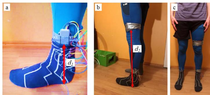
Fig. 2. Experimental setup: Position of the ankle (a) and tight (b) modules, initial position for measurements (c).
