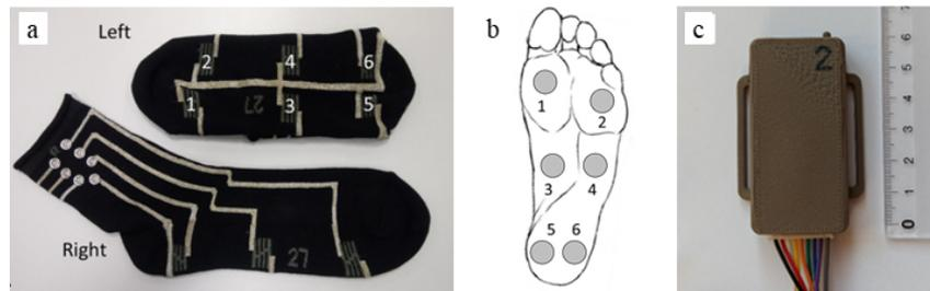
Fig. 1. Pair of dAid smart socks with knitted sensors marked by numbers (a); typical position of sensors over the foot plantar surface (b); data acquisition module (c).
