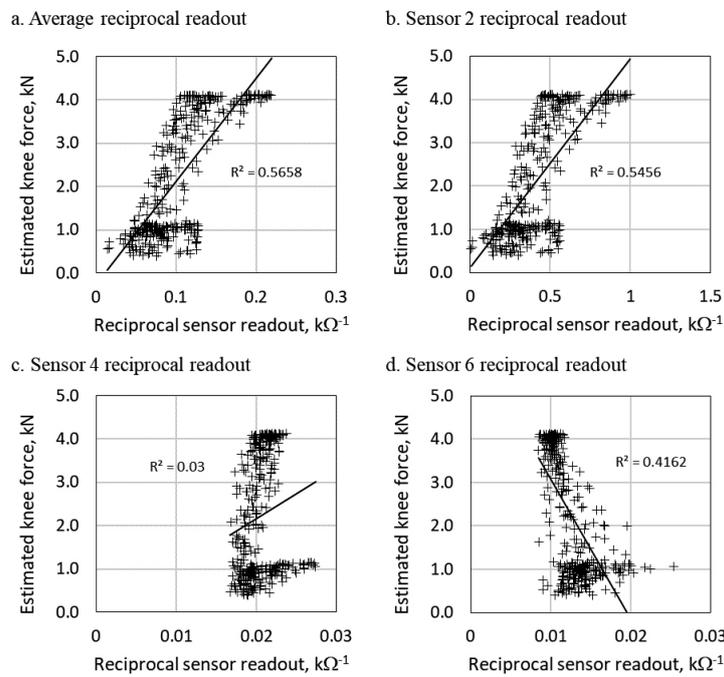
Fig. 5. The correlation diagram for the estimated knee joint force and reciprocal data of the selected sensors: a) averaged data; b) toe lateral sensor (Sensor 2); c) middle lateral sensor (Sensor 4); d) heel lateral sensor (Sensor 6).
