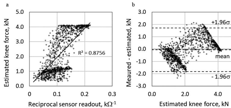
Fig. 6. Linear regression approximation for the estimated knee joint force (a) and corresponding Bland-Altman plot (b).
