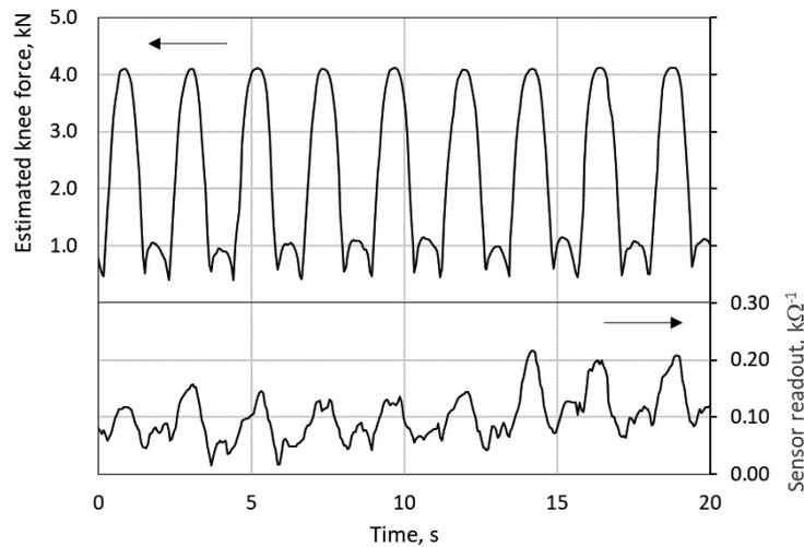
Fig. 4. The typical waveforms of the estimated knee joint force (top) and average reciprocal sock sensors readout (bottom) for a series of squats.
