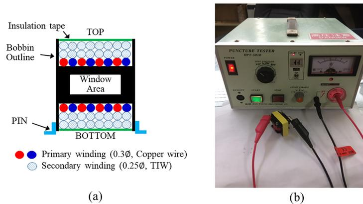
Fig. 2. Design and evaluation of the isolation transformer. a. Winding method of the primary and secondary side, b. Actual view of verification the insulation performance.
