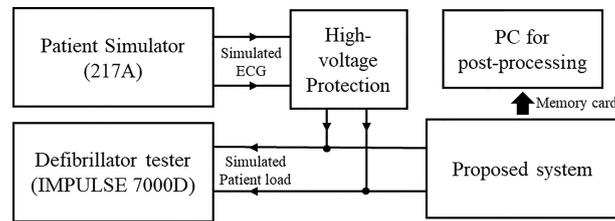
Fig. 3. Testing environment. The patient simulator generated an ECG signal and the defibrillator tester provided 50 Ω patient load.
