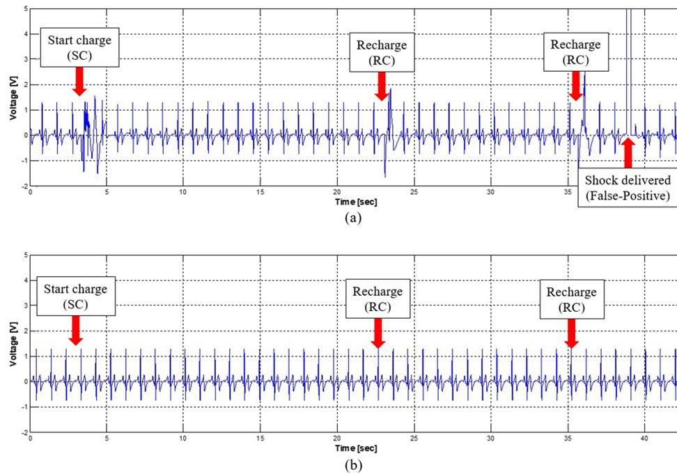
Fig. 5. Comparison of the ECG signal before and after application of the isolation barrier. a. Before the proposed method, False-Positive case occurred, b. Electrical noise was not induced and the diagnosis algorithm was operating normally.
