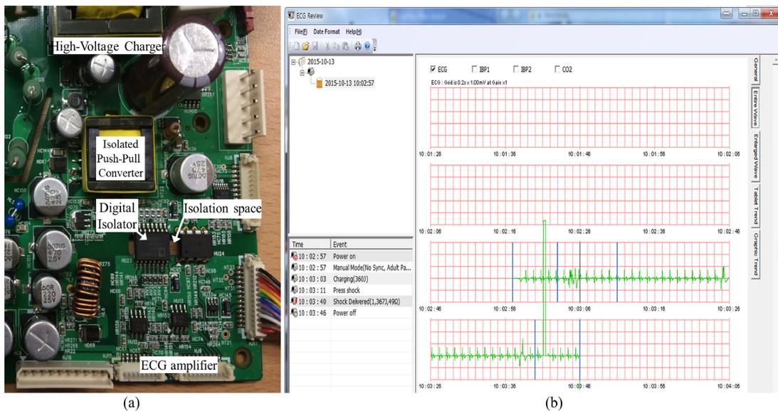
Fig. 4. A circuit with the proposed method and data plotting viewer. a. Actual view of the proto-type circuit, b. Custom-made electrocardiogram viewer.
