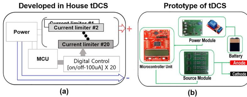
Fig. 1. (a) Block diagram of a developed in-house tDCS system, and (b) picture of a developed in-house tDCS system.
