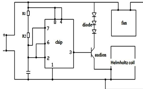
Fig. 1. PEMF circuit schematic diagram.
