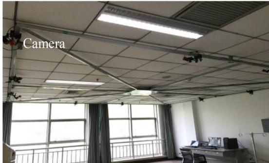
Fig. 1. Motion capturing system.
