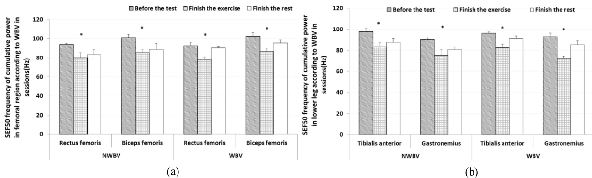
Fig. 4. Results of SEF 50 frequency of cumulative power for observing muscle fatigue according to WBV (mean \pm SD, *p < 0.05 ): (a) Femoral muscles, (b) Lower leg muscles.
