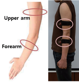
Fig. 8. Ideal attachment position of inertial measurement unit and real attachment position.
