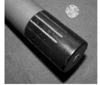
Fig.1: Prototype 16-electrode urethral probe. The diameter is 50 mm. The electrodes are of brass. Contact surface is 2x50mm2
