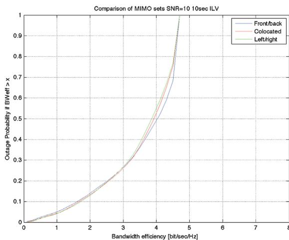
Fig. 23. Comparison of different antenna configurations.
