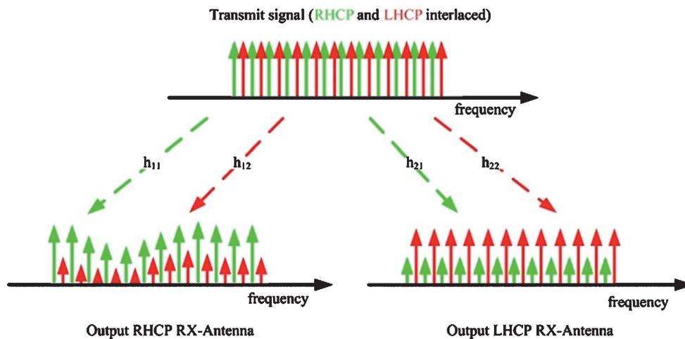
Fig. 7. Interlacing of RHCP and LHCP showing effects of transmission path ( $h_{11}$ ,  $h_{22}$  co-polarized transmission,  $h_{12}$ ,  $h_{21}$  cross-polarized transmission).
