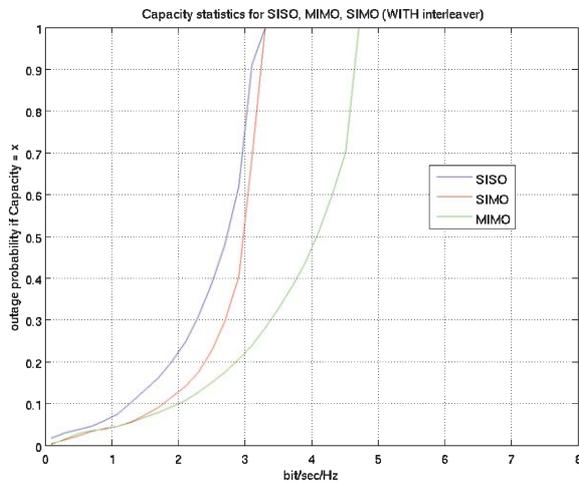
Fig. 22. Outage probability with time interleaving (10 sec).
