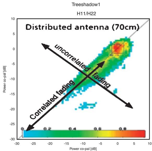
Fig. 17. Correlation of fading, antenna distance approx. 70 cm.
