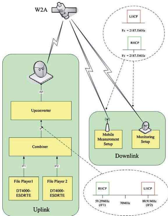
Fig. 6. Overview to the measurement setup.
