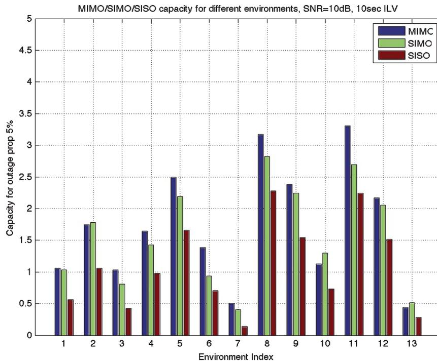
Fig. 24. Estimated capacity for different environments, SNR = 10 dB.
