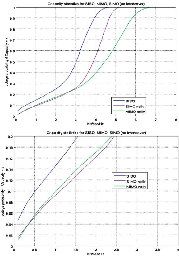
Fig. 21. Outage probability versus capacity, “instantaneous capacity” (= no interleaving), environment “sub-urban2”.
