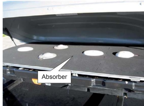
Fig. 4. Antenna assembly used for measurement campaign #1.
