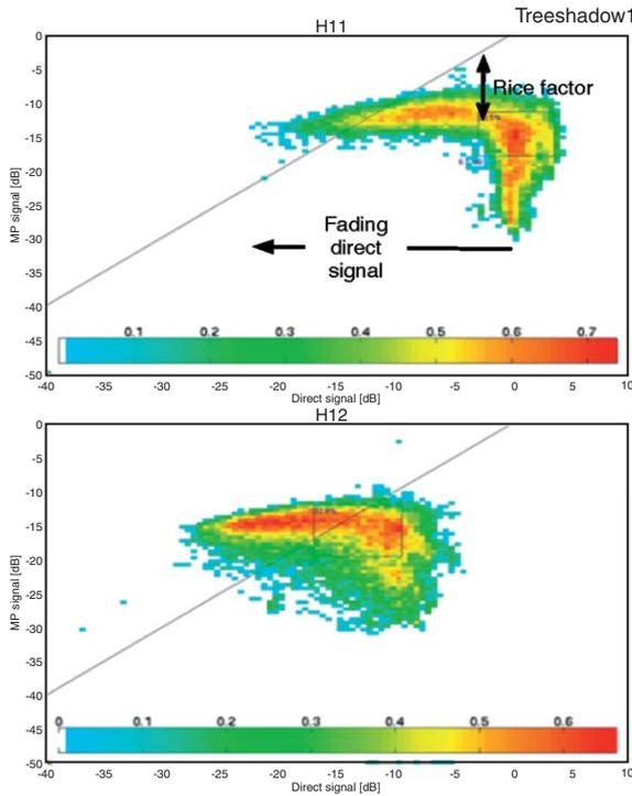
Fig. 20. Impact of the fading to the XPD
