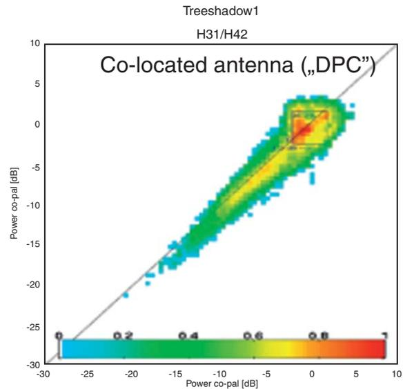
Fig. 18. Correlation of the fading, “co-located” antenna.
