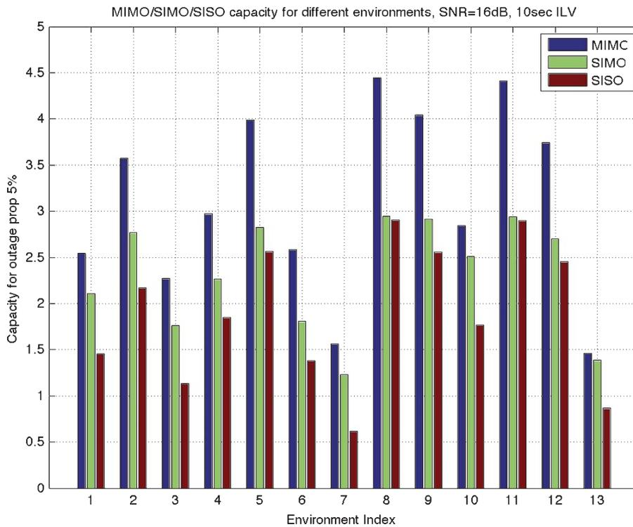
Fig. 25. Estimated capacity for different environments, SNR = 16 dB.
