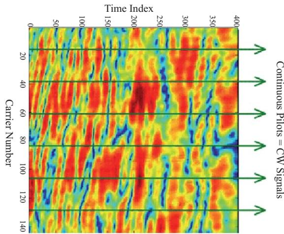
Fig. 10. Example of wideband recording of an OFDM signal showing the placement of continuous pilot signals.
