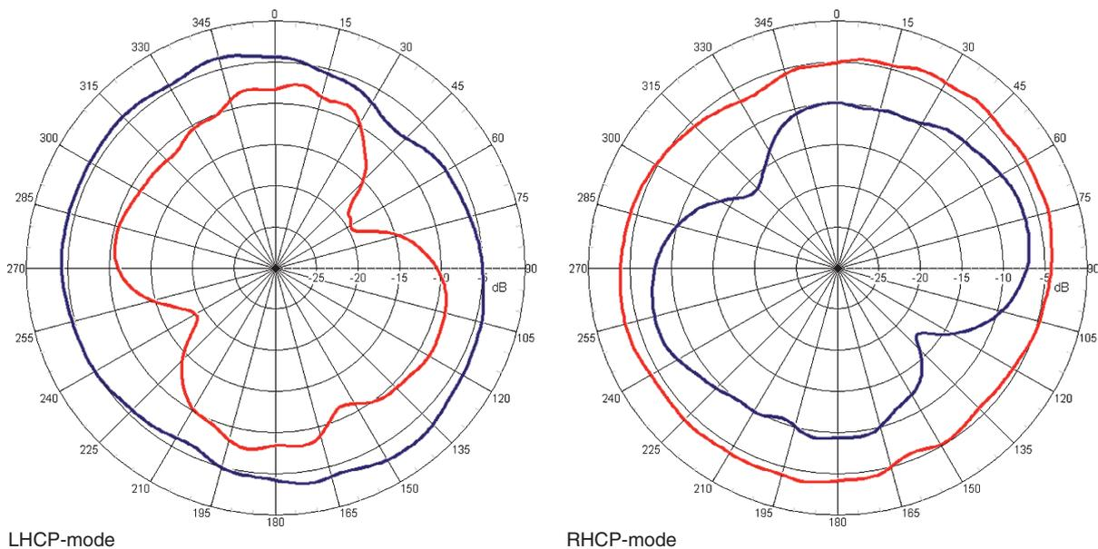
Fig. 5. Antenna patterns for FhG DPC antenna (Theta: 60°, frequency 2185 MHz; red crosspol signal, blue copol signal).
