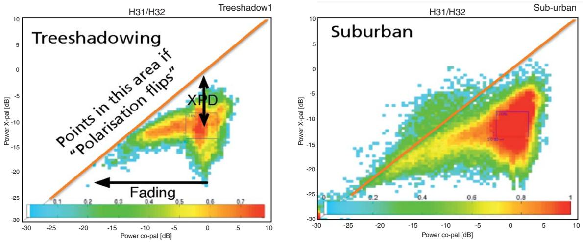
Fig. 19. Impact of the fading to the XPD.
