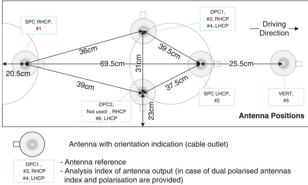
Fig. 3. Position of antennas of the MIMOSA antenna array on groundplane.
