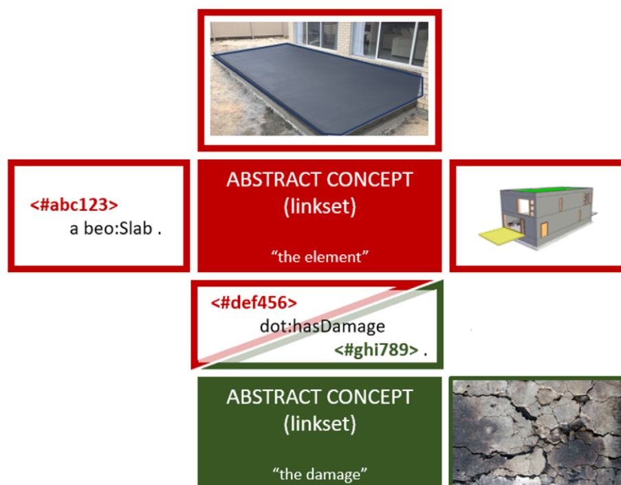
Fig. 4. Document-specific representations of two concepts. Any relationships between those concepts will also be expressed via representations, i.e., the concepts themselves will not be enriched directly with project data.
