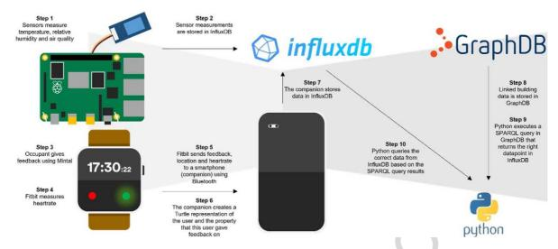
Fig. 2. Experimental setup to integrate occupant feedback with linked building data.
