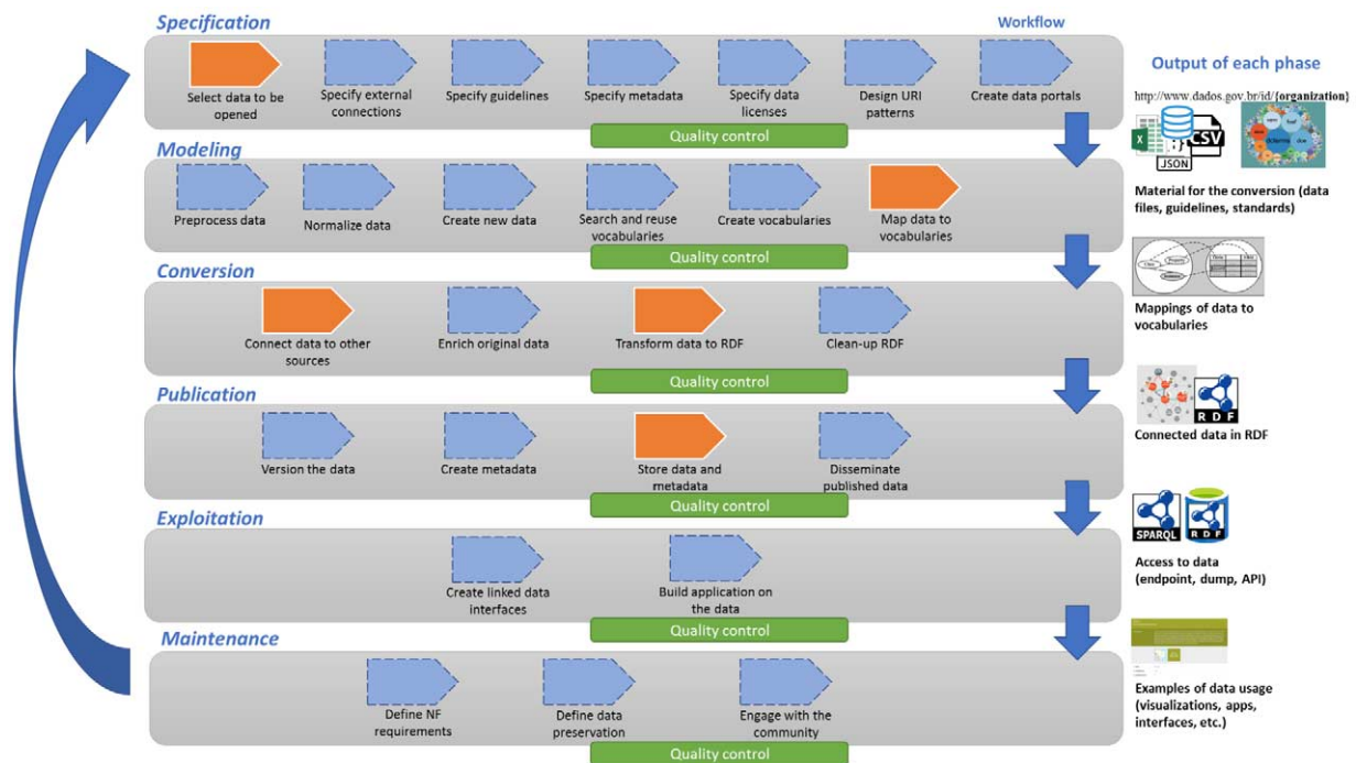
Fig. 5. Unified process model proposed in this paper. The sequence of tasks flow from left to right, up to bottom. In orange, the mandatory tasks for having linked data, in blue, the optional tasks. Adapted from [70].
