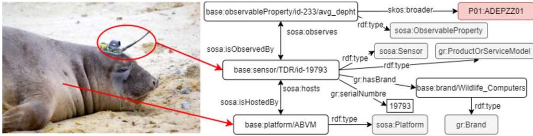
Fig. 1. SES platform and TDR sensor description.
