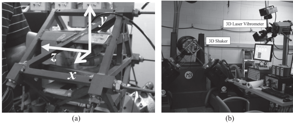
Fig. 2. The test setup for the measurement of glove transmissibility spectra on the fingers in the three orthogonal directions (3-D: x , y , and z ) using a 3-D laser vibrometer [21]. (a) a gloved hand on the instrumented handle. (b) the layout of the test equipment.
