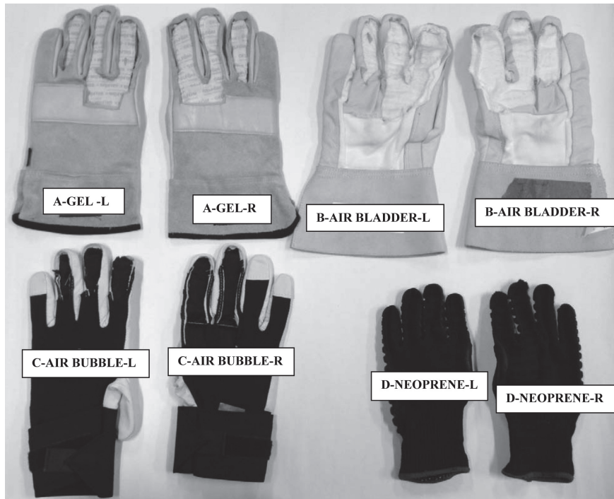
Fig. 1. Four types of VR gloves (two for each type) considered in this study: Glove A – thick gel pad; Glove B – air bladder with pump; Glove C – cellular air bubbles; and Glove D – dipped neoprene.
