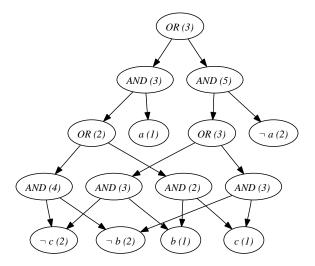
**Figure 2.** The DAG of the d-DNNF formula  $(a \land ((b \land c) \lor (\neg b \land \neg c))) \lor (\neg a \land ((b \lor \neg c) \lor (\neg b \lor c)))$ . Each node in this graph is also labeled with the value used to compute the minimum cardinality of the root.
