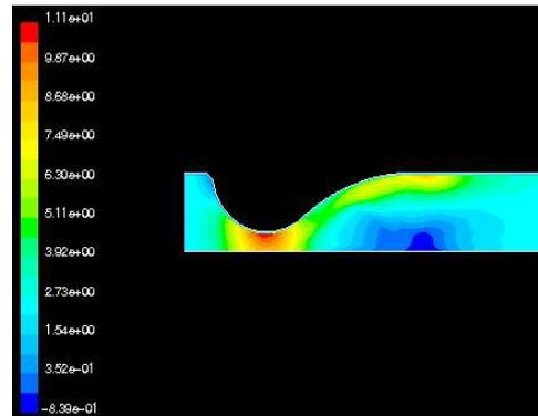
Fig. 2. Mean velocity contours [k-ε model].
