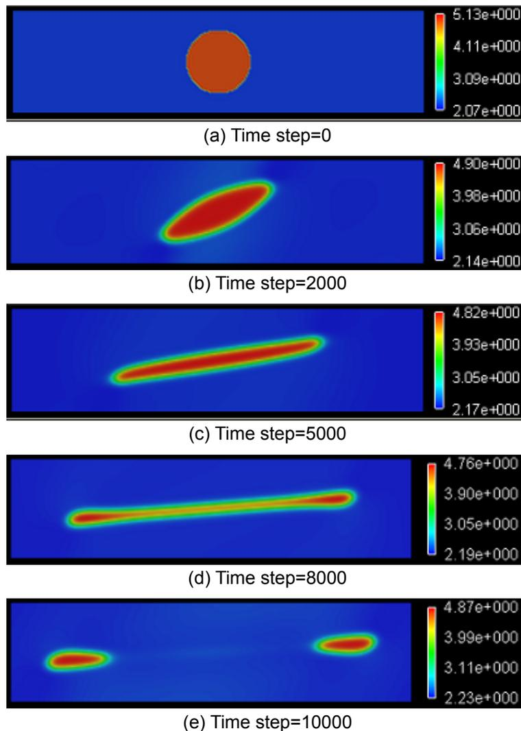
Fig.1. The droplet breaking in a shear flow.
