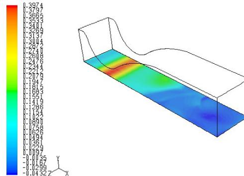
Fig. 4. Bottom wall shear stress [LES model].
