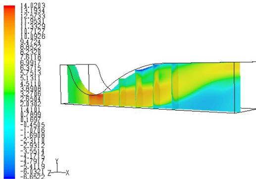
Fig. 3. X direction velocity contours [LES model].
