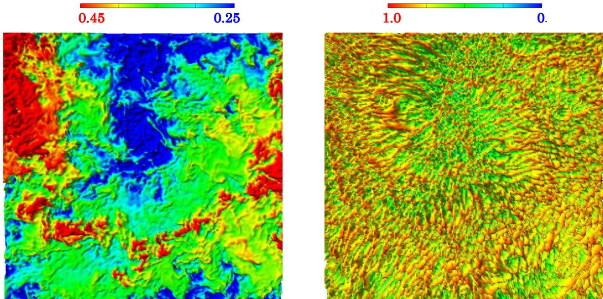
Fig. 1. Instantaneous temperature fields in the central vertical plane ( $z/D=0.5$ )-left and deeply inside thermal boundary layer ( $z/D=0.001$ )-right, for highly turbulent thermal convection of air between two infinite horizontal plates,  $Ra=10^9$ ,  $Pr=0.71$ .
