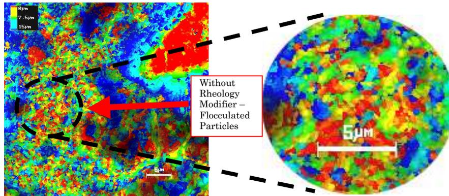
Fig. 1. Three dimensional representation of simulated high level nuclear waste without rheology modifier.
