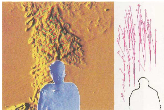
Fig. 19. Natural convection around a human body (correlation method).
