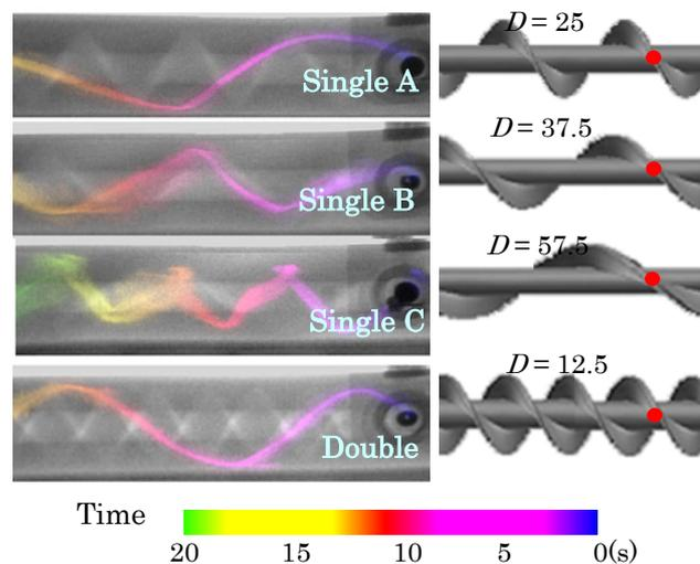
Fig. 4. The color path lines of powder flow.
