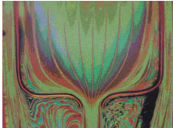
Fig. 4. It looks like the cocktail filled in a rolling cup [Original caption: A two-dimensional sink (Gharib, M. & Bezaie, M. 1999)].
