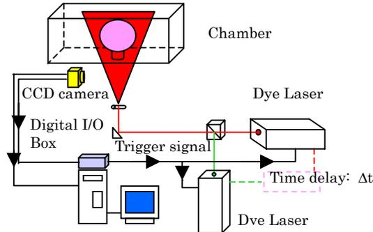
Fig. 1. PIV system for bubble collapse flow.
