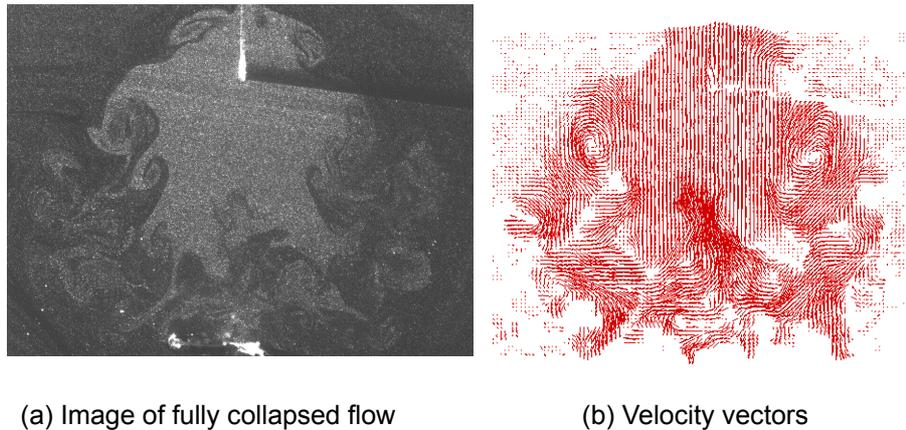
Fig. 8. Soap bubble fully collapsed flow.
