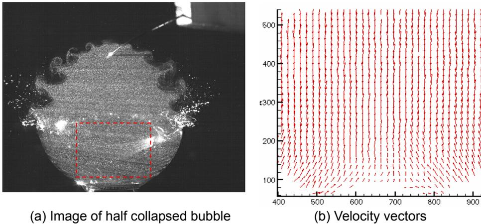
Fig. 6. Measurements of a half collapsed soap bubble.
