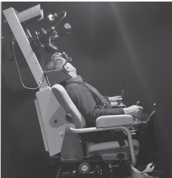
Fig. 1. Subject seated in the computerized rotational head impulse test (crHIT) device. The subject is seated in the LARP testing position, which requires the LARP plane to be earth-horizontal because the axis of rotation of the crHIT device is earth-vertical.
