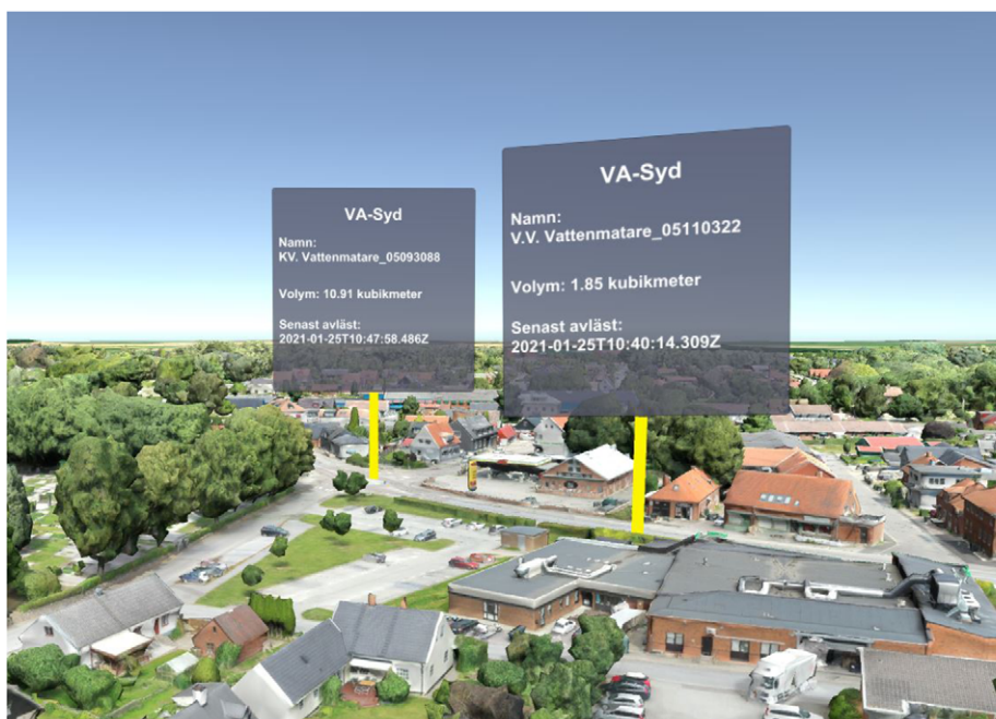
Fig. 3. The “digital tvilling” in Veberöd village – a water consumption monitor system. Source: https://smartabyar.se/ (photo used with permission from Byutveckling AB).
