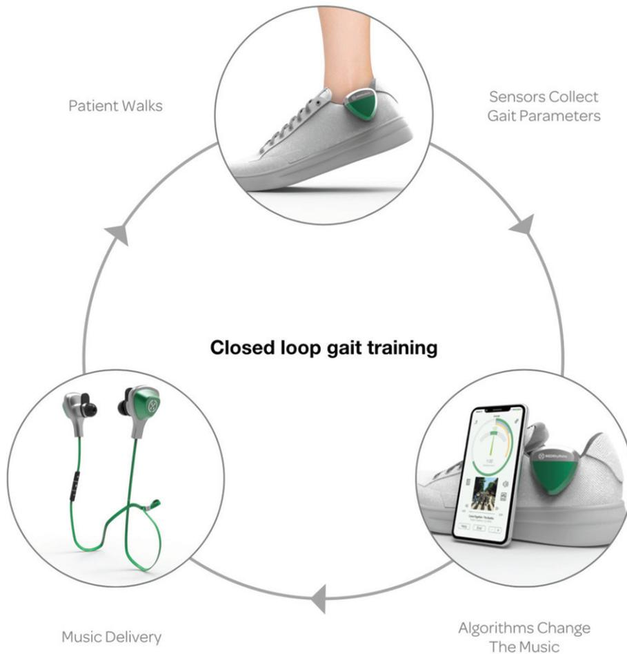
Fig. 1. Digital Closed Loop Gait Training Therapeutic In the top portion of the figure, a sensor is worn on the shoe to collect real-time walking cadence. A smartphone (lower right) houses the music playlist and delivers the acoustic signals through headphones worn (lower left) by the patient. Algorithms time shift the music to match the patient's cadence and modulate according to entrainment outcomes.
