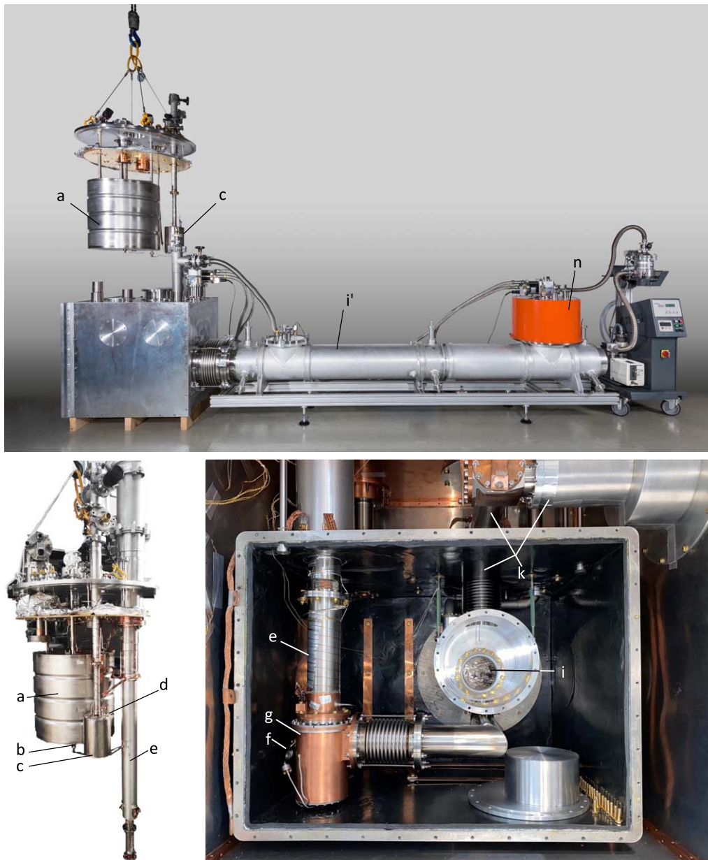
Fig. 2. Pictures of SuperSUN with the same labeling as in Fig. 1: (a) the 100 L liquid helium bath, (b) the needle valve, (c) the 1-K pot, (d) the superleak, (e) the ^3\text{He} pumping column, (f) the ^3\text{He} impedance, (g) the ^3\text{He}/^4\text{He} heat exchanger, (i) the superfluid conversion volume, (i') vacuum vessel containing the thermally screened conversion volume, (k) the UCN extraction system, (n) the 4-K cryostat. Credit top photo: Ecliptique – Laurent Thion.
