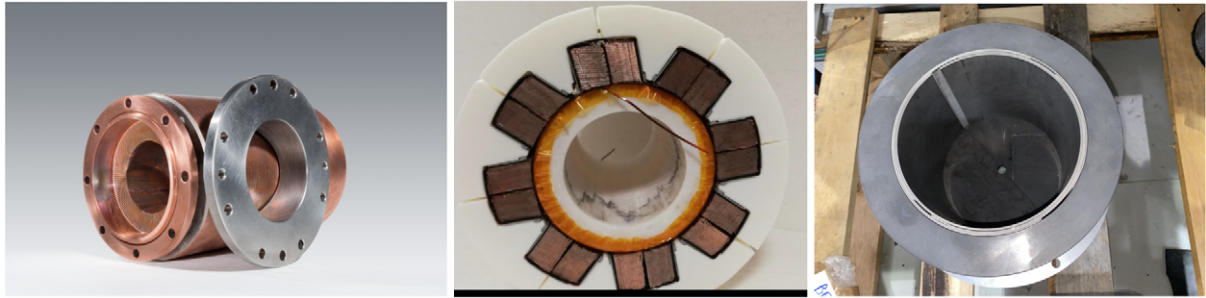
Fig. 3. Left: picture of the {}^3\text{He}/{}^4\text{He} heat exchanger, credit: Ecliptique – Laurent Thion. Middle: picture of a cut through a mockup of the octupole superconducting magnet. Right: picture of the beam-dump.
