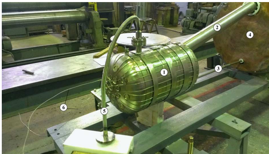
Fig. 11. UCN converter vessel mockup (1 – helium vessel, 2 – helium vapor pipe, 3 – He-II supply pipe, 4 – heat screen, 5 – wire pipe, 6 – 250 Ohm nichrome electrical heater). The He-II vessel has a diameter of 300 mm and a length of 500 mm. The chamber is equipped with a helium level gauge and a temperature sensor.
