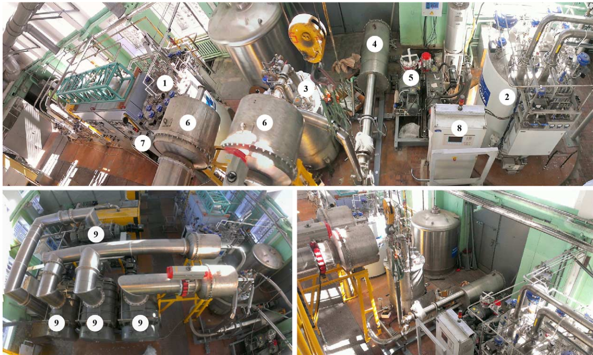
Fig. 10. UCN source mockup at the WWR-M reactor (1 – helium liquefier L-280; 2 – helium refrigerator TCF-50; 3 – helium cryostat; 4 – UCN source model; 5 – pumping unit for isotopically pure ^4\text{He} gas; 6 – helium vapor heaters; 7 – liquefier control cabinet; 8 – refrigerator control cabinet; 9 – helium roots pumps).
