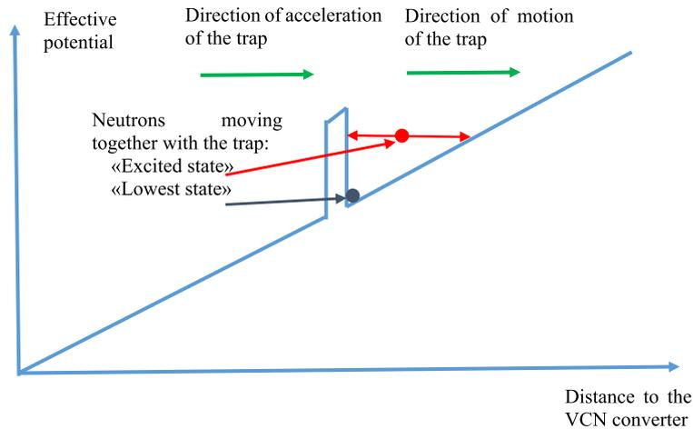
Fig. 4. Effective potential locking the neutron bunch in the coordinate system associated with the running-away accelerating trap.
