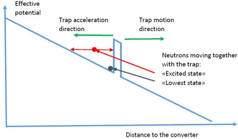
Fig. 2. Effective potential that traps the neutron bunch in the reference system associated with the runaway decelerating trap.
