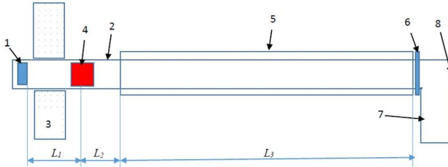
Fig. 1. A scheme of the installation to produce and accumulate UCNs: 1 – VCN converter, 2 – specular guide, 3 – biological shielding of the neutron source, 4 – time focusing device, 5 – segment of deceleration of VCNs to UCNs, 6 – fast valve, 7 – UCN accumulation volume, 8 – thin separating foil.
