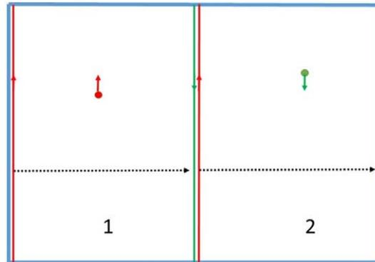
Fig. 3. A simplified illustration of the principal possibility of doubling the UCN density by adding UCNs with opposite polarization directions in one volume. The storage volume is shown with thick blue line. Magnetized foils can slide along the inner walls, shown by red and green lines with arrows.
