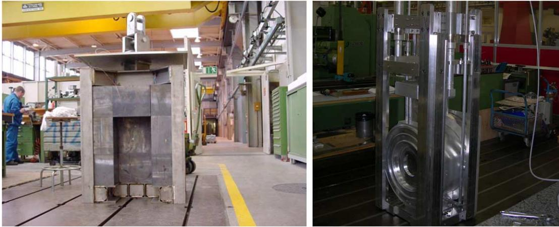
Fig. 2. Left: Target #1, composed of a water-cooled pile of lead bricks [2]. Right: Target #2, consisting in a water-cooled lead cylinder [9].
