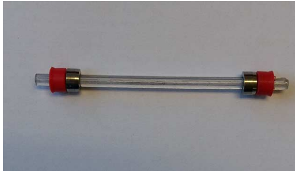
Fig. 3. Sapphire capillary with 3 mm outer diameter and 1 mm inner diameter. The capillary is installed into the housing by pressing the seals with forces parallel to the capillary so that there are no torsion forces on the capillary.
