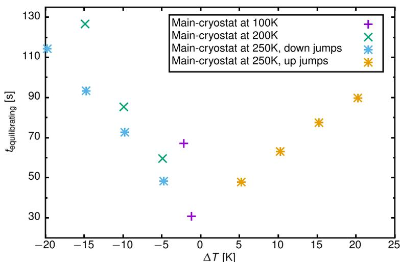
Fig. 6. Time to reach the final sample temperature to within 0.1 K at different temperature jump sizes ( $\Delta T$ ) and different main cryostat temperatures. The sub-cryostat was in all cases mounted under vacuum inside a CCR cryostat. The largest  $|\Delta T|$  for each series indicates the largest possible jump which can be achieved with the given base temperature (see Fig. 5(a) for an example of the limits at lowest temperature).
