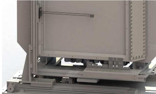
Fig. 7. CAD of the beam stop device with respect to the detector, and the beamstop parking area located outside of the detector sensitive area. The dimensions of the beam stops are according to Table 1.
