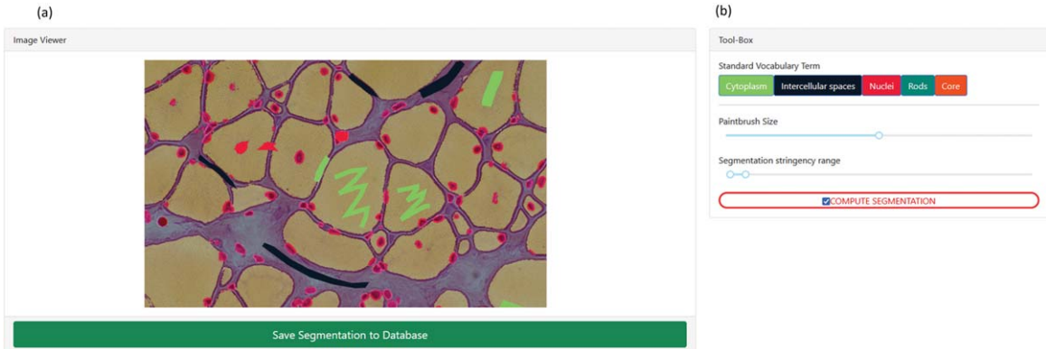
Fig. 6. Screenshot of the image annotation module. (a) Image viewer used to navigate, zoom and annotate the histology image. (b) Menu interface to select the annotation label, brush width and segmentation parameters.
