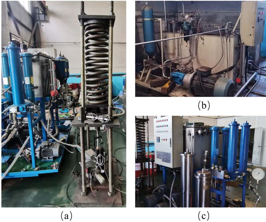
Fig. 8. Valve-controlled hydraulic cylinder system. (a) Valve-controlled hydraulic cylinder. (b) Former hydraulic oil pump. (c) Latter hydraulic oil pump.
