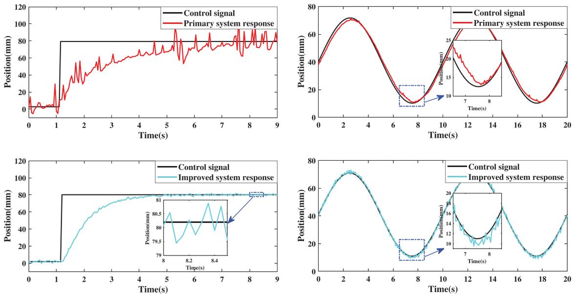
Fig. 9. Performance test results of the primary system and the improved system. (a) Step response. (b) Sine response.
