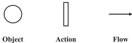
Fig. 2. Graphical representation of D-Petri Net.
