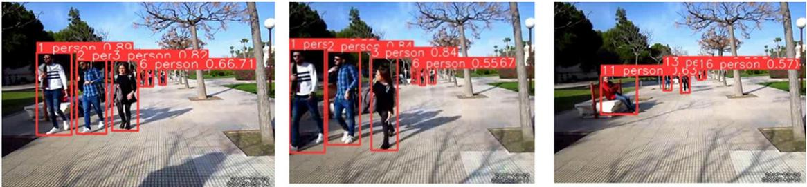
Fig. 7. Results of pedestrian detection using YOLOv5 on three frames taken from the video dataset.
