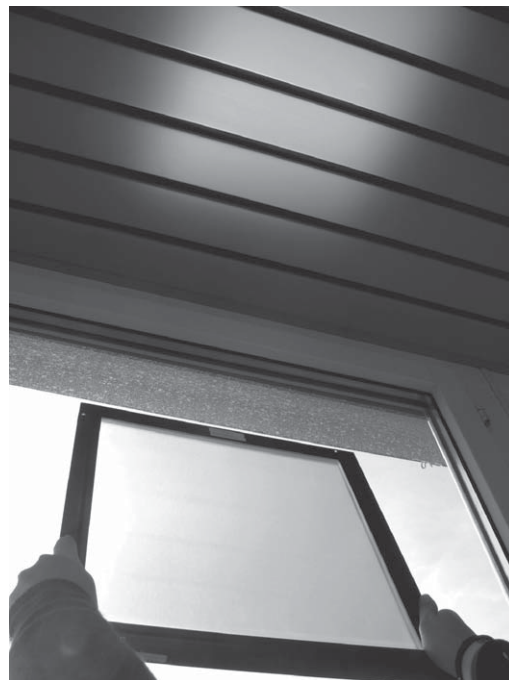
Fig. 9. Sample glass plate with a layer of the micro-structured film used in our case study held against a window on a sunny day, showing both the redirection effect on the ceiling and the reduced transmission for the direct view through the sample.
